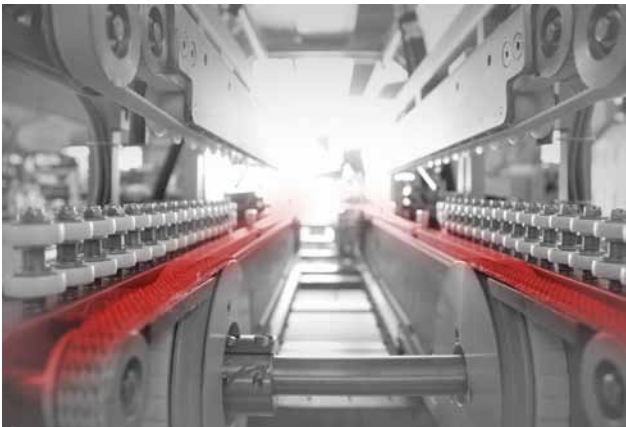
Image 4 The path for a cardboard packaging cycle. It is initially folded, then filled and finally sealed.
